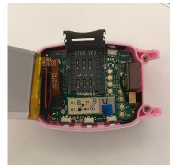
Figure 9. To install a SIM card in the Gator 2, you first have to disassemble the watch.
